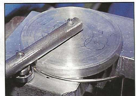
8. The removable line guard is shaped in a vice.
