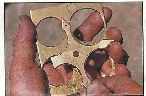
7. The starback feature for the Avon Classic four and a half inch model is cut from brass plate, then turned on the lathe and finished by hand.
