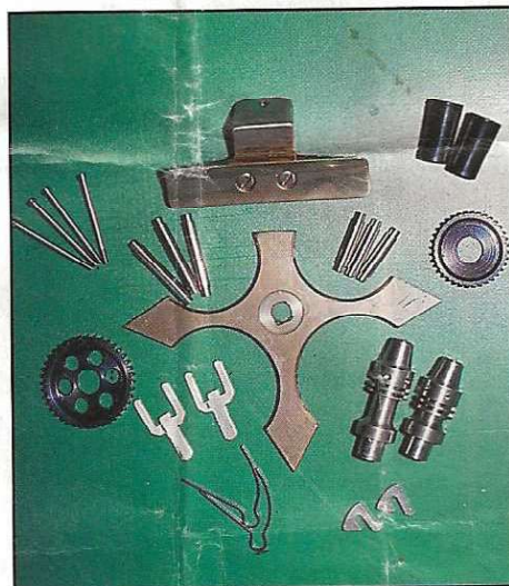
6. Whilst anodising is in progress, the 45 component and precision parts such as the centre bush, spokes and reel seat are manufactured and made ready for assembly on the return of the plates.
